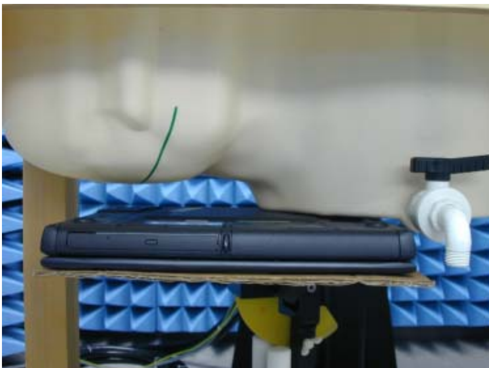
Fig.5 Photograph of the top cover parallel and at a distance of 0.0 cm from the base of the phantom
