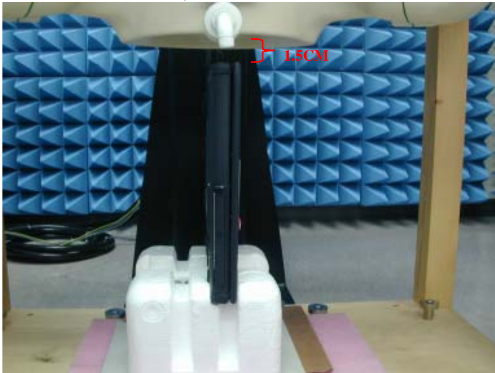
Fig.4 Photograph of the edge of the PC at 90° and at a distance of 1.5 cm from the base of the phantom
