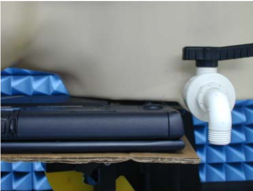
Fig.6 Photograph of the top cover parallel and at a distance of 0.0 cm from the base of the phantom
