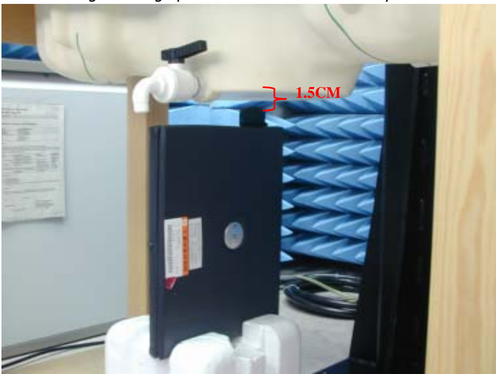
Fig.3 Photograph of the edge of the PC at 90° and at a distance of 1.5 cm
