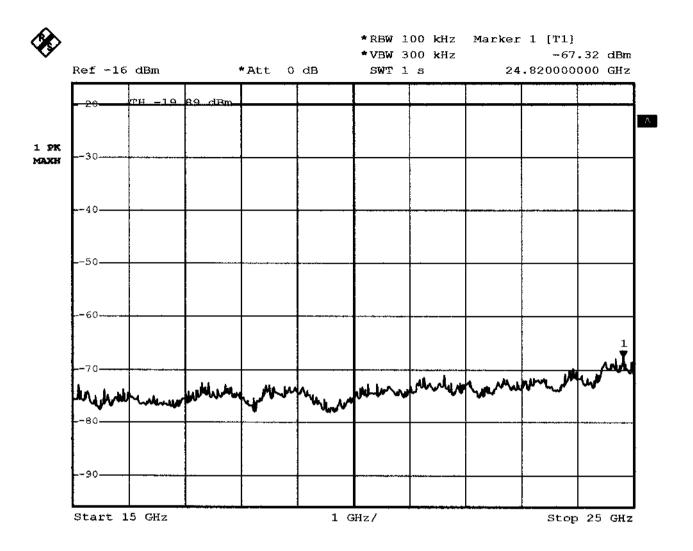
Comment A: RF conducted spurious at middle channel external att.=3dB cable loss=1dB
