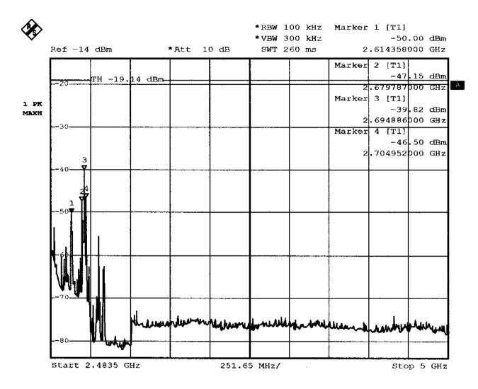
Comment A: RF conducted spurious at low channel external att.=3dB cable loss=1dB
