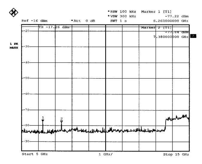
Comment A: RF conducted spurious at high channel external att.=3dB cable loss=1dB
