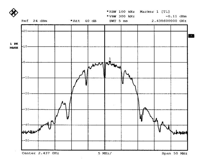
Comment A: RF conducted spurious at middle channel external att.=3dB cable loss=1dB
