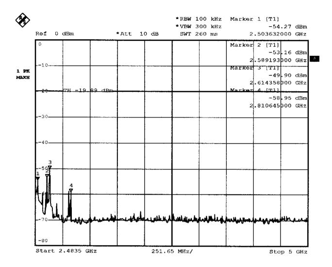
Comment A: RF conducted spurious at middle channelre external att.=3dB cable loss=1dB
