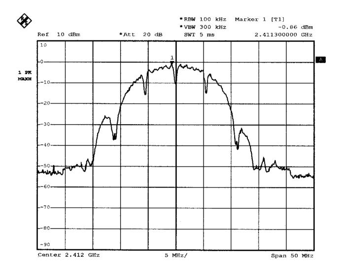
Comment A: RF conducted spurious at low channel external att.=3dB cable loss=1dB
