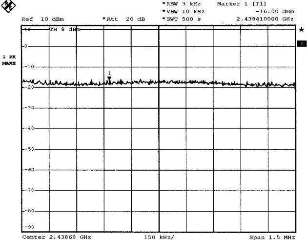
Comment A: Power density at middle channel external att.=3dB cable loss=1dB
