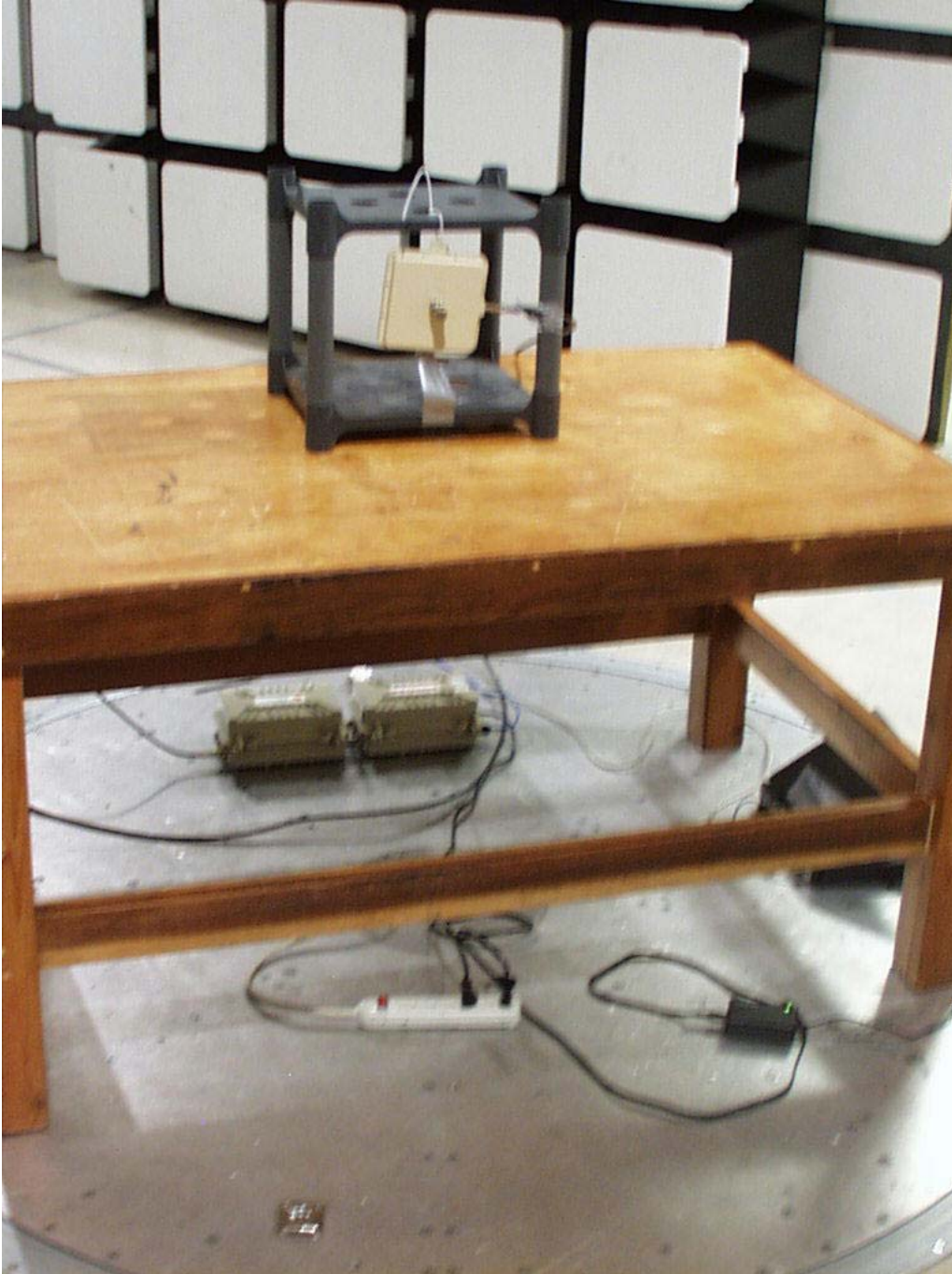
EUT (ODU) radiated test set-up
