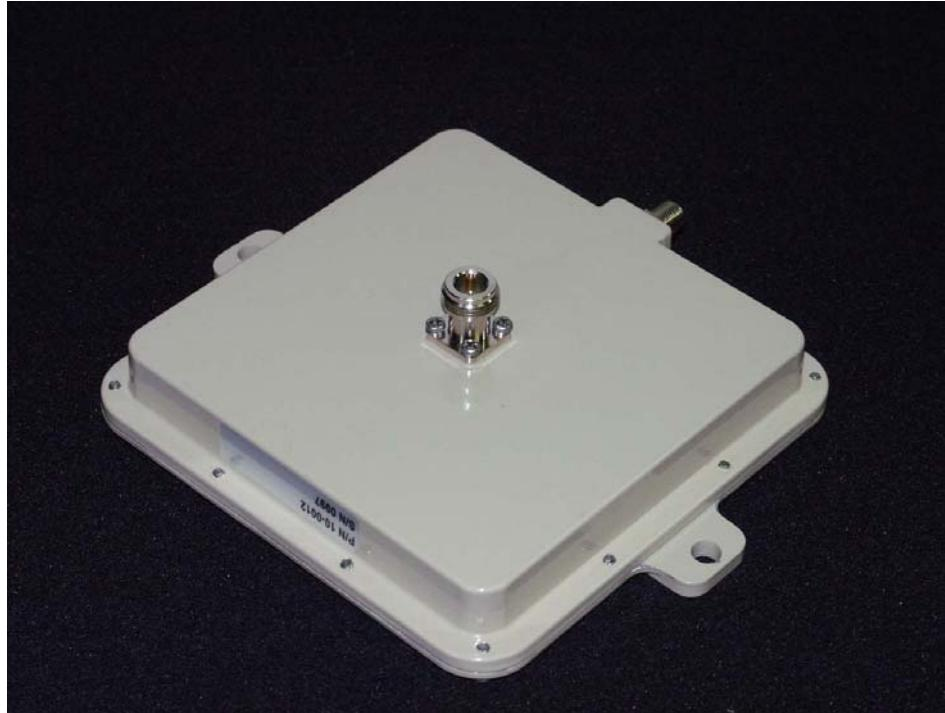
The Transceiver unit functions as the RF interface for both the Base Station (BTS) and the CPE Modem endpoints. The Transceiver can be configured with various antenna gain combinations and models and is powered over the single connecting RF cable by either the CPE Modem or the BTS.
