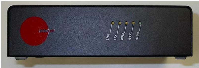
The Customer Premise Equipment (CPE) Modem functions as the endpoint user interface to the Internet or other media types. The CPE is an easily configurable subscriber Modem unit. That provides a 10BaseT connection type for multiple applications such as Data, Voice, and Video. The CPE is partnered with a Power supply that operates at 110VAC or 220VAC.
