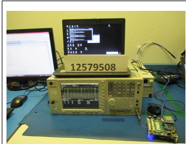
RF ANTENNA PORT CONDUCTED
