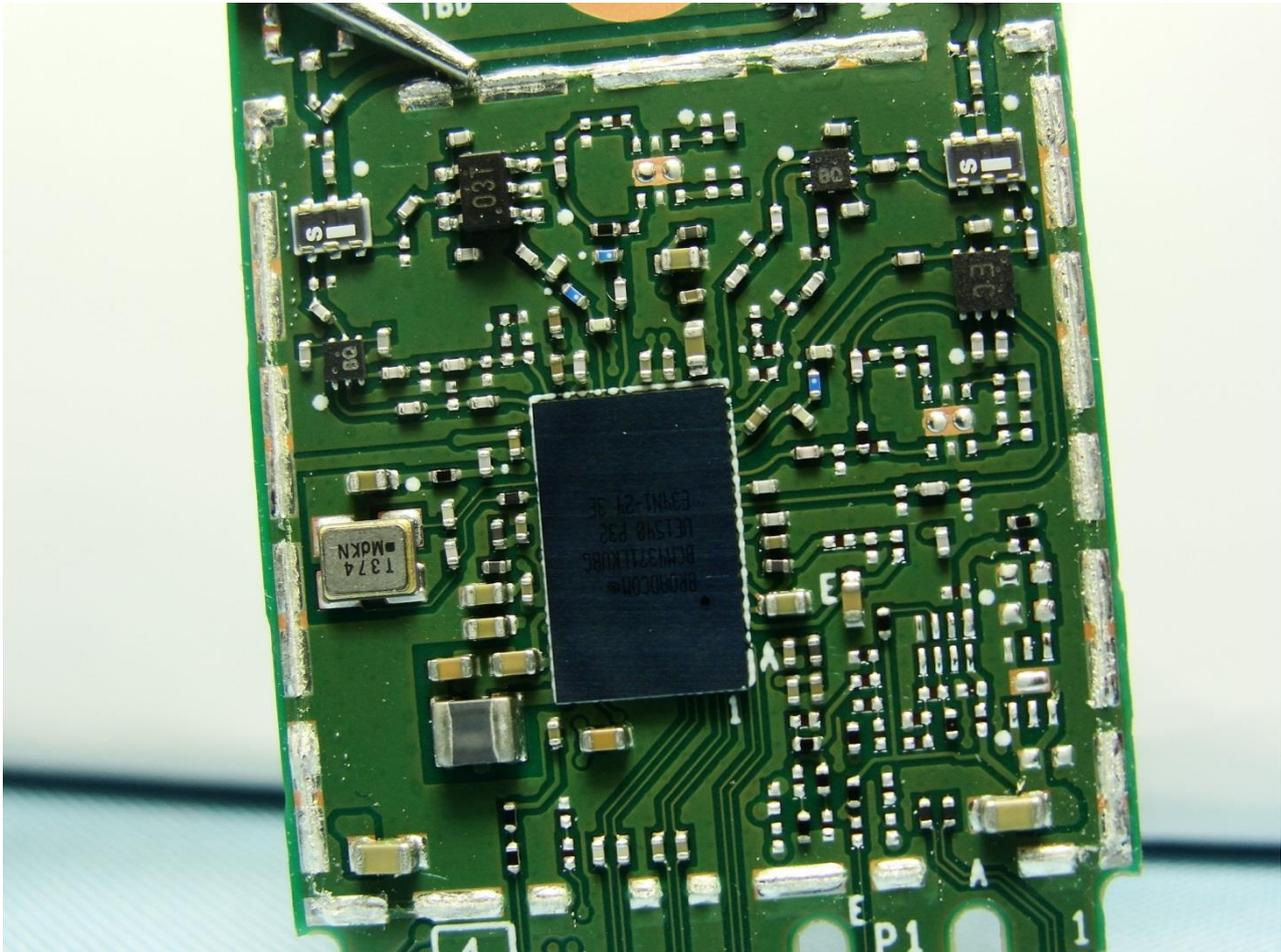
EUT: Broadcom 802.11 a/b/g/n/ac WLAN + Bluetooth PCI-E/SDIO NGFF 2230 Card
