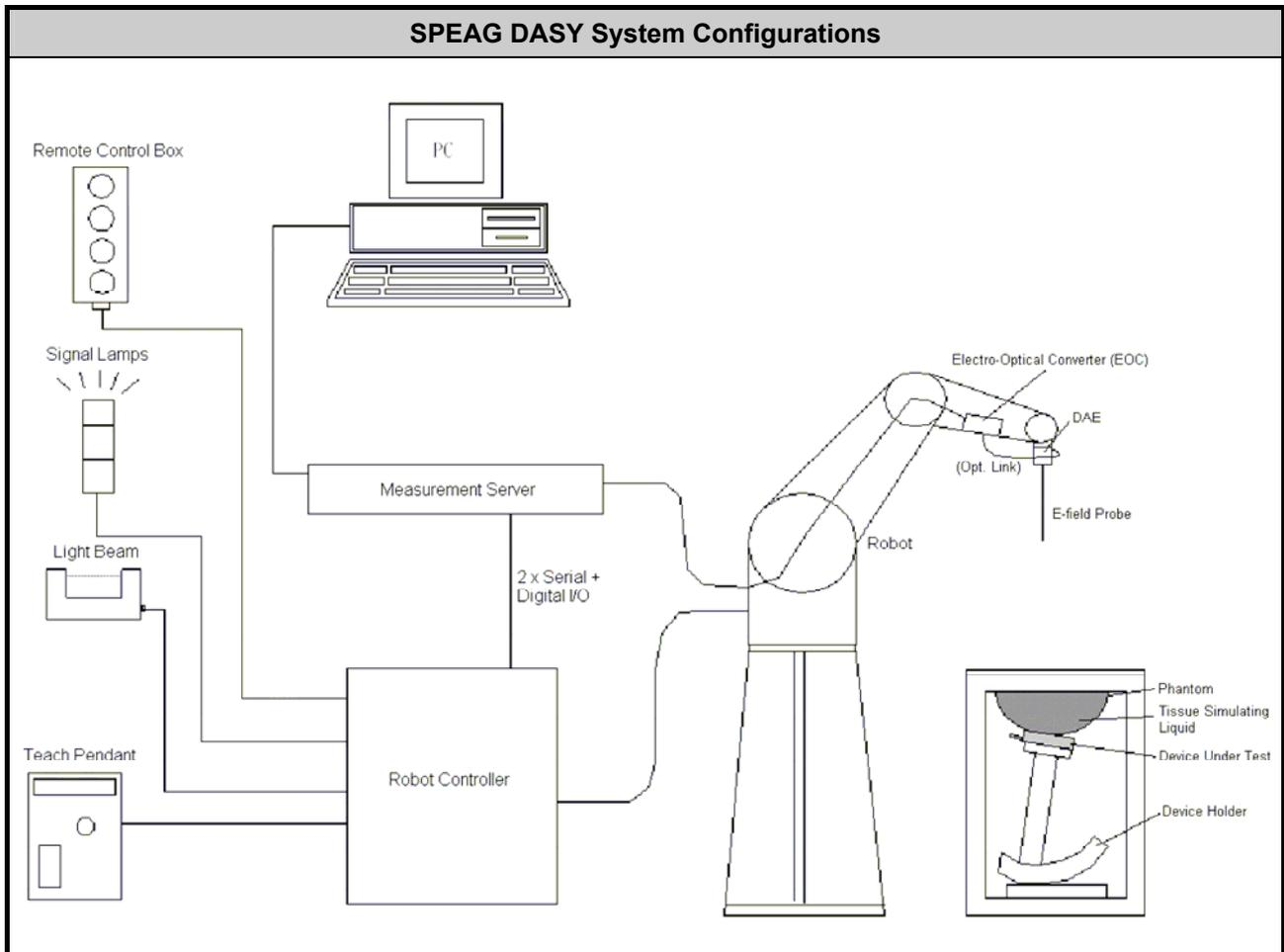
The DASY system for performance compliance tests is illustrated above graphically. This system consists of the following items:
