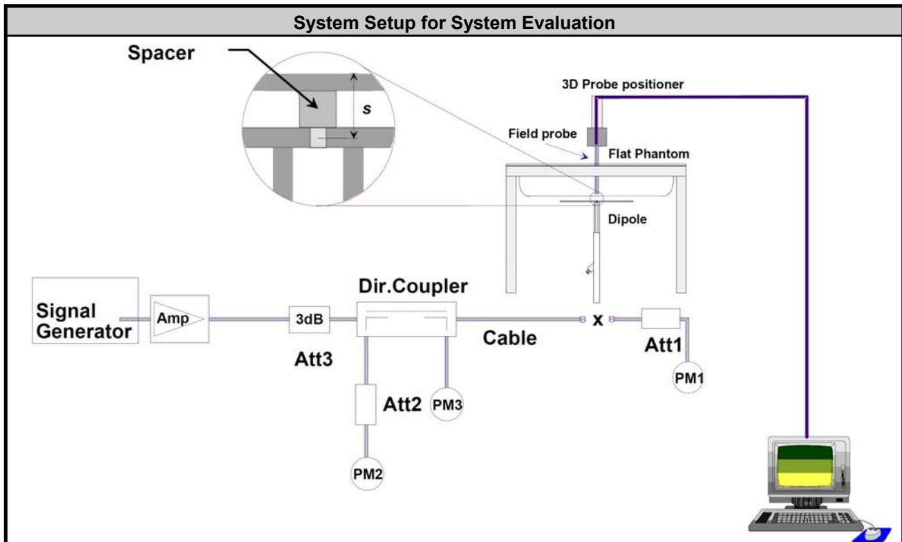
**Photo of Dipole Setup**
