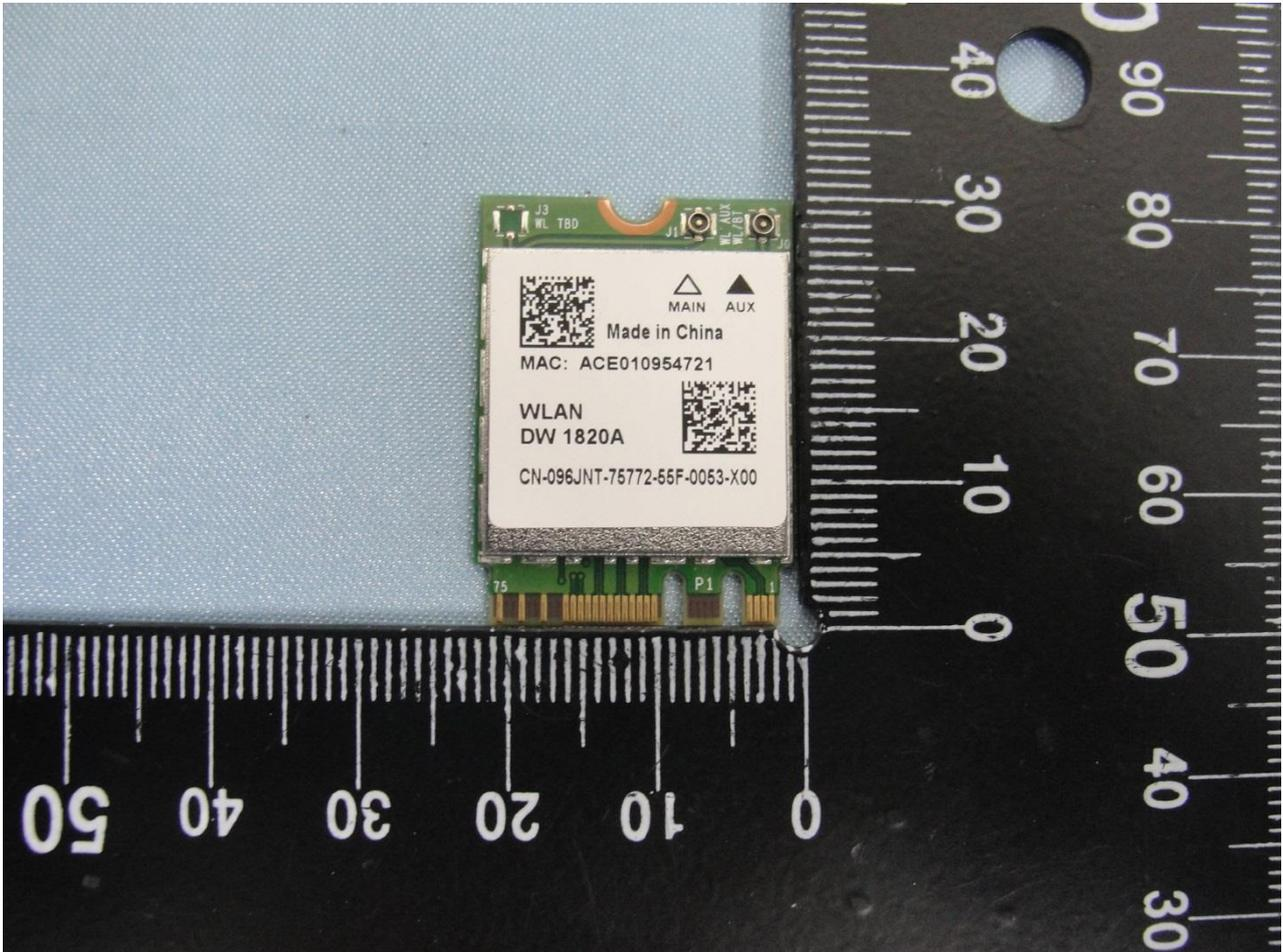
EUT: 802.11b/g/n/a/ac WLAN + Bluetooth PCI-E NGFF 2230 Card
