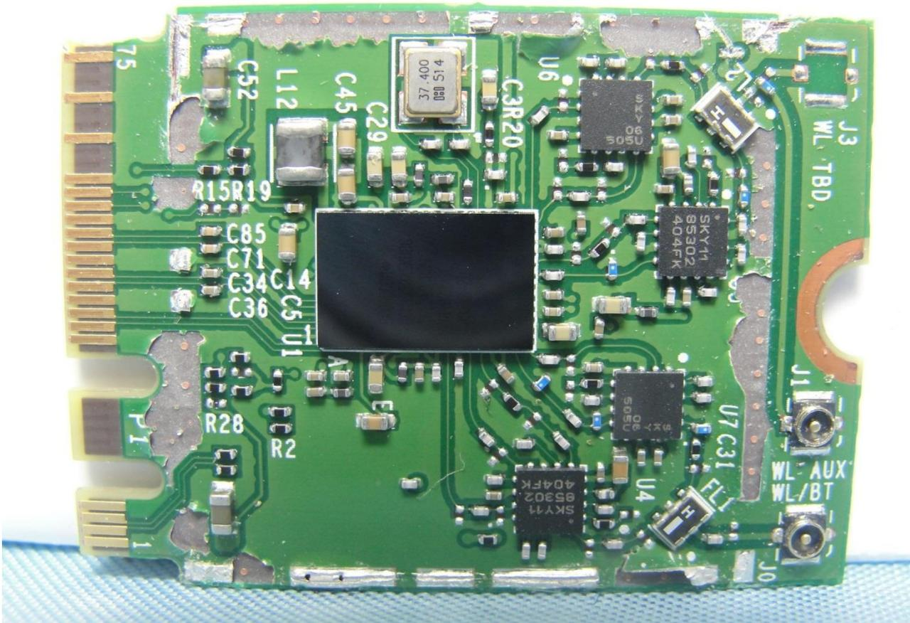
EUT: 802.11b/g/n/a/ac WLAN + Bluetooth PCI-E NGFF 2230 Card
