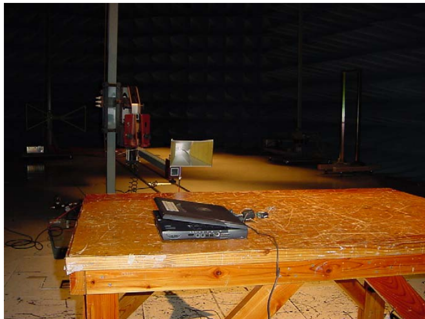
Photograph 3. Radiated Emission Test Setup 1-26GHz
