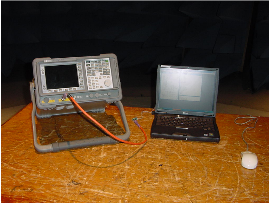
Photograph 6. Conducted Measurements Setup
