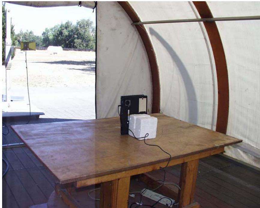
**POWERLINE CONDUCTED EMISSIONS MEASUREMENT SETUP**
