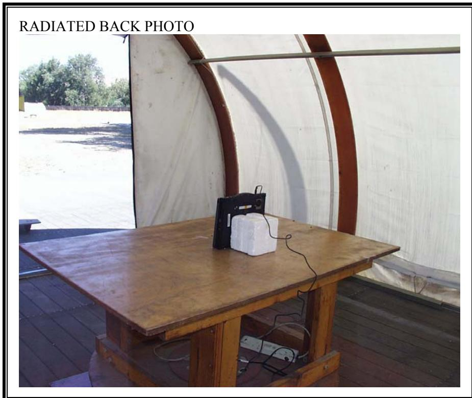
**RADIATED RF MEASUREMENT SETUP – Z Configuration**
