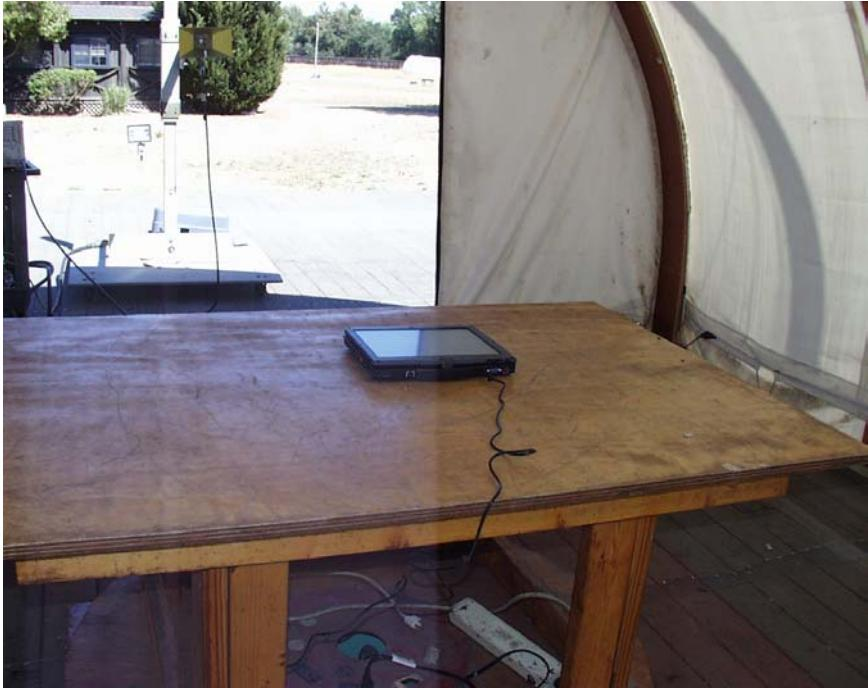
**RADIATED RF MEASUREMENT SETUP – Y Configuration**
