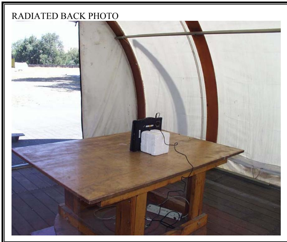
**RADIATED RF MEASUREMENT SETUP – Z Configuration**
