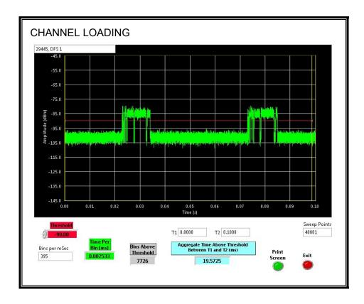
The level of traffic loading on the channel by the EUT is 19.57%
