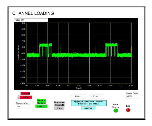
The level of traffic loading on the channel by the EUT is 21.55%
