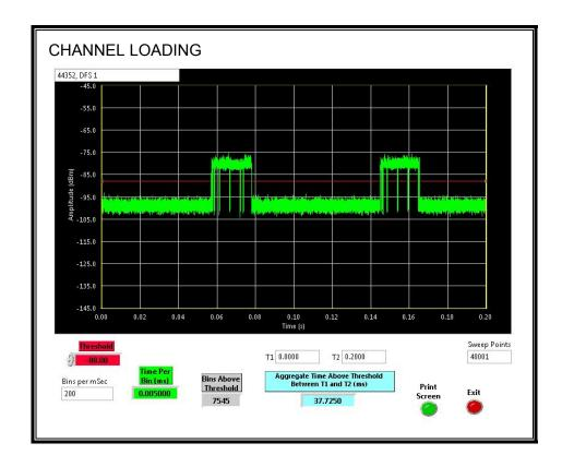
The level of traffic loading on the channel by the EUT is 18.86%
