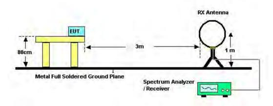
For Radiated Emissions: 30MHz~1GHz
