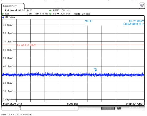
Plot on Configuration For EDR (8DPSK) / Hopping / 2483.5MHz~2500MHz (down 20dBc) (Vertical)
