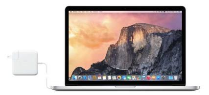
Charge the battery. Connect your MacBook Pro to a power outlet using the included cable and 60W (13-inch model) or 85W (15-inch model) MagSafe 2 Power Adapter. The battery recharges more quickly when the computer is shut down or in sleep.
