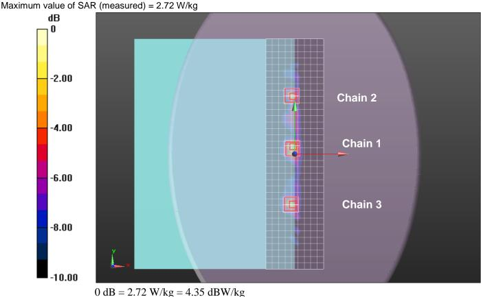
Frequency: 5785 MHz; Duty Cycle: 1:1; Room Ambient Temperature: 24.0°C; Liquid Temperature: 23.0°C Medium parameters used: f = 5785 MHz;  $\sigma$  = 5.87 S/m;  $\epsilon_r$  = 47.83;  $\rho$  = 1000 kg/m<sup>3</sup> DASY5 Configuration:
