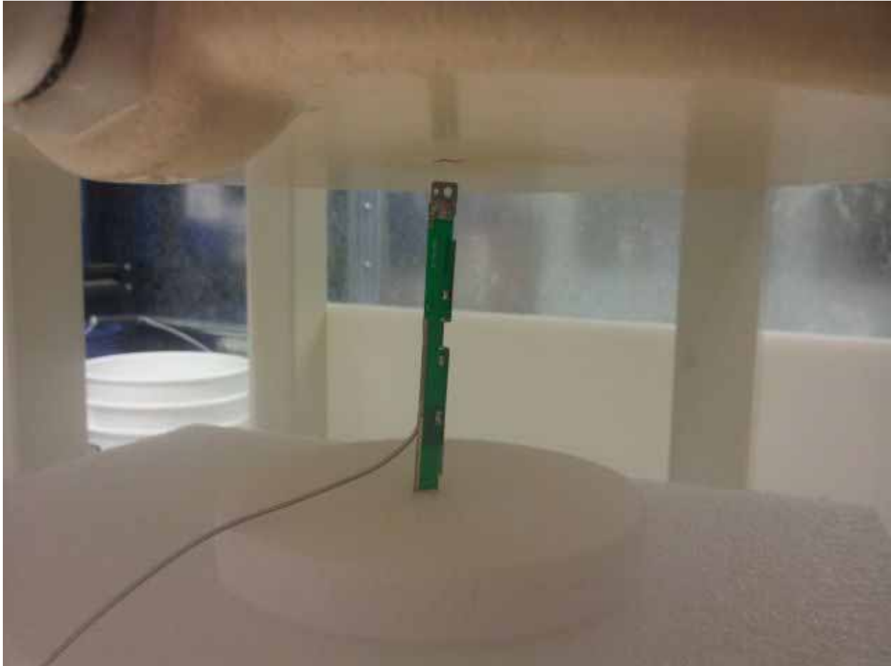
Picture 6: ACON APP8P-700045 antenna, Orientation = Top
