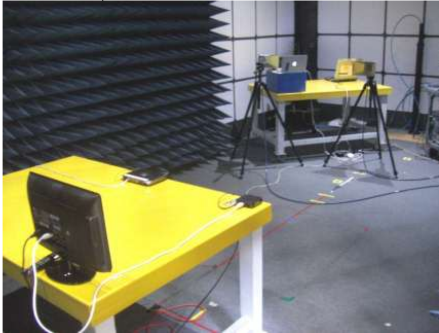
DFS FRONT PHOTO (CLIENT-TO-CLIENT COMMUNICATIONS MODE SETUP)
