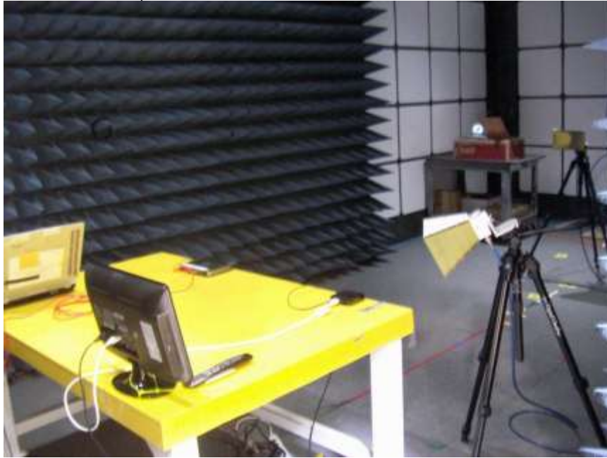
DFS FRONT PHOTO (CLIENT-TO-CLIENT COMMUNICATIONS MODE SETUP)
