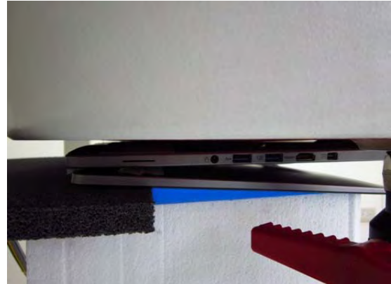
Fig.3 EUT Lap-held mode to flat phantom
