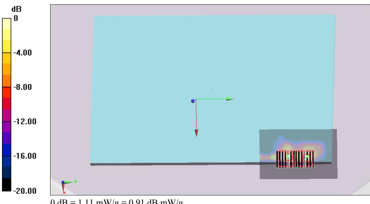
**#09\_WLAN5G\_802.11n-HT20 MCS0\_Bottom Face\_0cm\_Ch52;Ant MIMO****DUT: 13-2-347**
