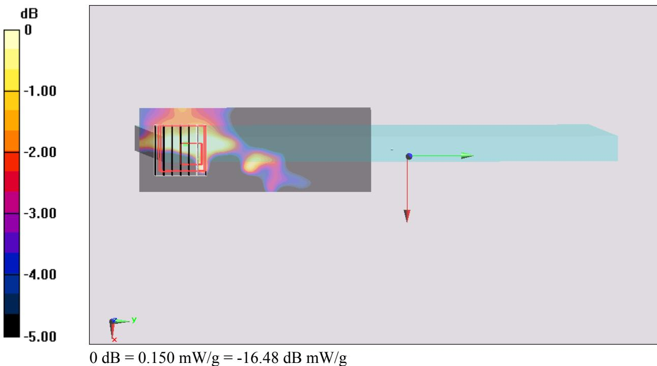
**#04\_WLAN5G\_802.11n-HT20 MCS0\_Curved surface of Edge1\_0cm\_Ch36;Ant MIMO****DUT: 13-2-351**
