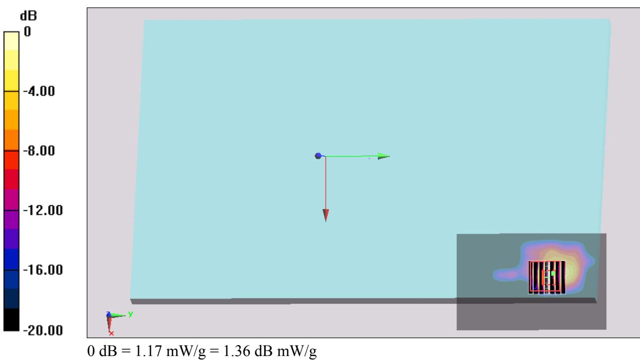
**#06\_WLAN5G\_802.11n-HT20 MCS0\_Bottom Face\_0cm\_Ch36;Ant MIMO****DUT: 13-2-351**
