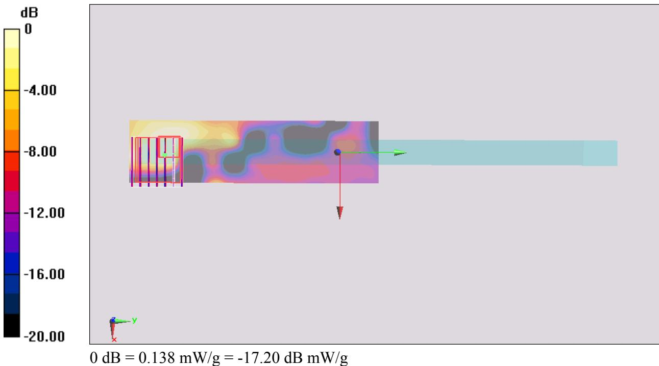
**#07\_WLAN5G\_802.11n-HT20 MCS0\_Curved surface of Edge1\_0cm\_Ch52;Ant MIMO****DUT: 13-2-351**
