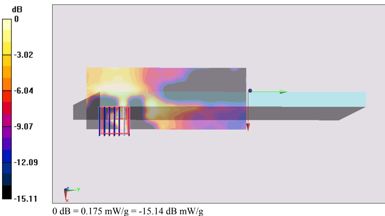
**#01\_WLAN5G\_802.11n-HT20 MCS0\_Curved surface of Edge1\_0cm\_Ch157;Ant MIMO****DUT: 13-2-351**
