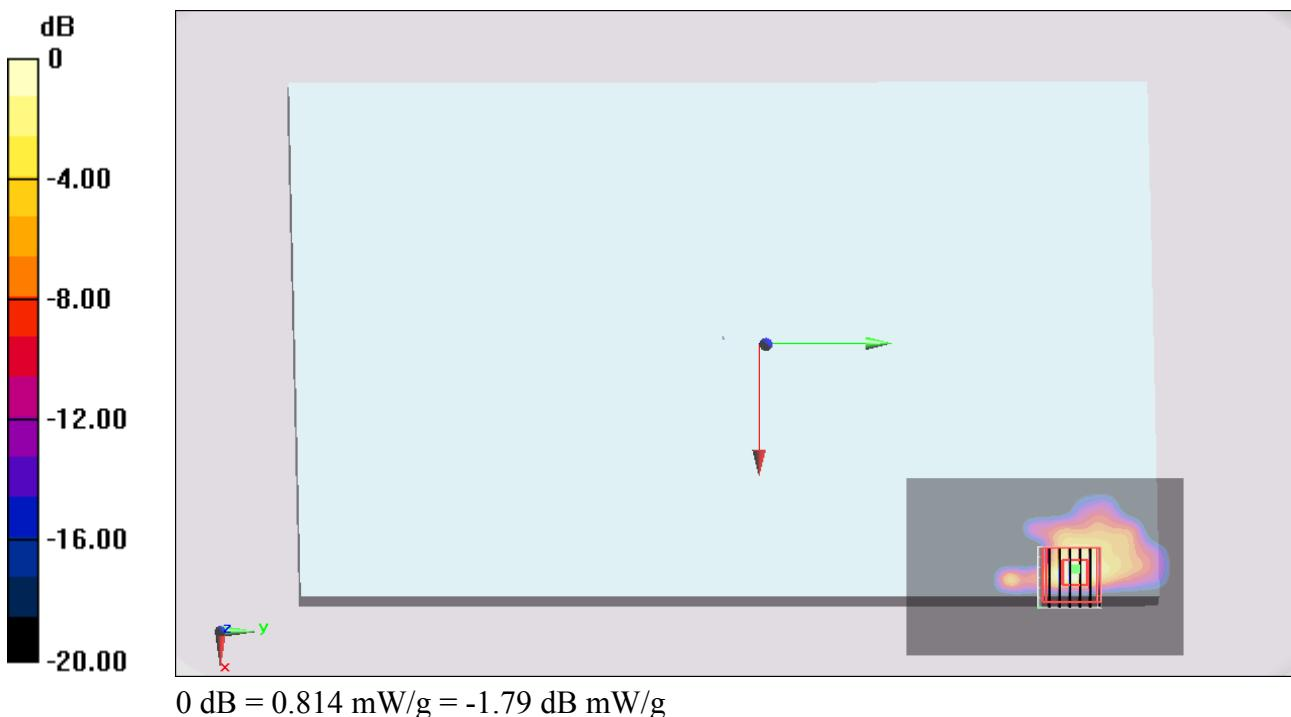
**#90\_WLAN5G\_802.11a 6Mbps\_Bottom Face\_0cm\_Ch64;Ant Main****DUT: 13-2-347**
