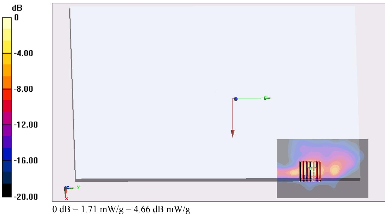
**#16\_WLAN5G\_802.11n-HT20 MCS0\_Bottom Face\_0cm\_Ch116;MIMO****DUT: 13-2-347**
