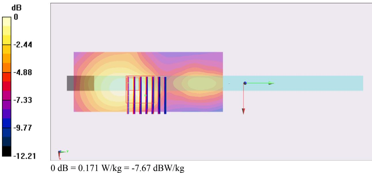
**#99\_WLAN2.4G\_802.11b 1Mbps\_Curved surface of Edge1\_0cm\_Ch1;Ant MIMO****DUT: 13-2-347**
