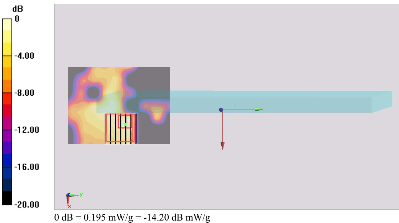
**#35\_WLAN5G\_802.11a 6Mbps\_Curved surface of Edge1\_0cm\_Ch165;Ant Main****DUT: 13-2-347**
