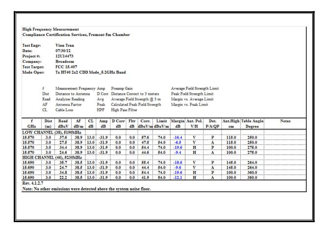
Note: tested with highest output powers at 17dBm to cover 1TX and STBC 2TX.
