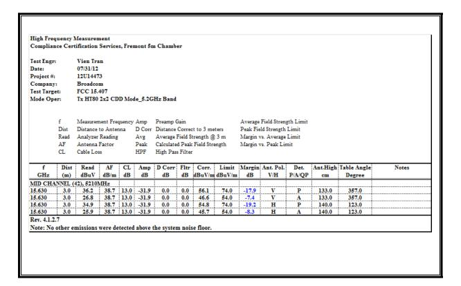
Note: tested with highest output powers at 17dBm to cover 1TX.
