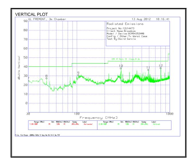
REPORT NO: 12U14473-3A EUT: 802.11a/b/g/n/ac WLAN + Bluetooth PCI-E Mini Card
