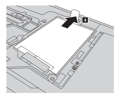
7 Take out the hard disk drive secured in a metal frame 5.
