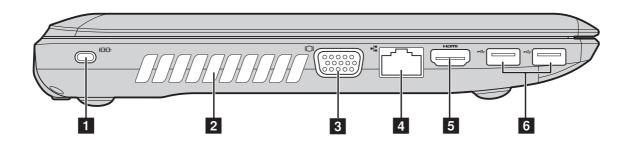
**Kensington slot** Attach a security lock (not supplied) here.
