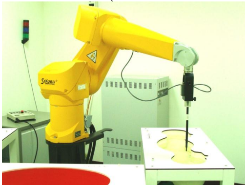
Fig 5.5 Photo of DASY4
