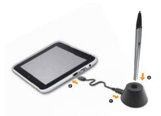
The digitizer pen is not fully charged at purchase. Charge the digitizer pen before using it for the first time. To charge the digitizer pen, do the following:
