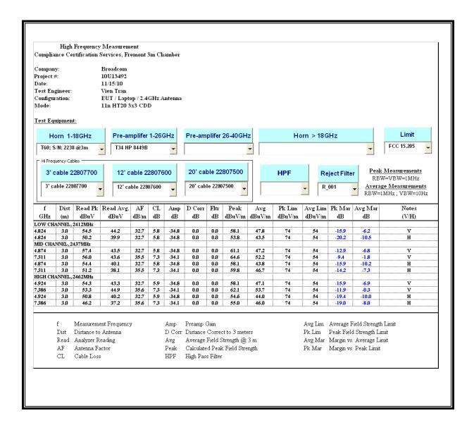
Test with the highest output power of g-mode mid channel as worst case for this mode HT20 3x3 CDD.
