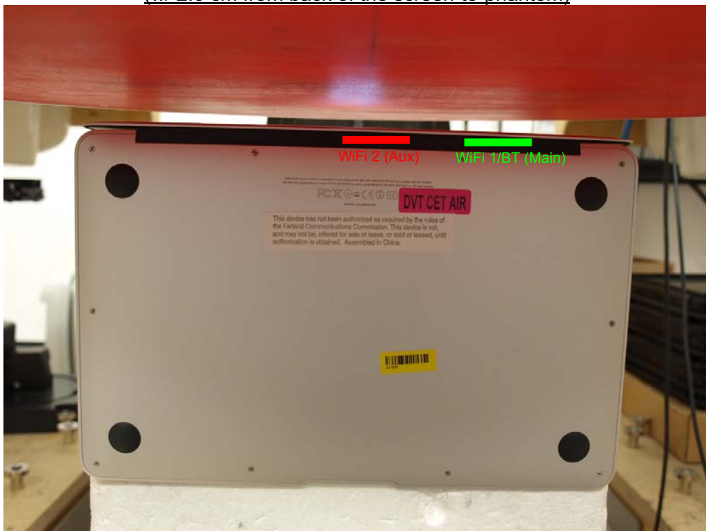
Nearby Person configuration for 11 inch MacBook Air (w/ 2.0 cm from back of the screen-to-phantom)
