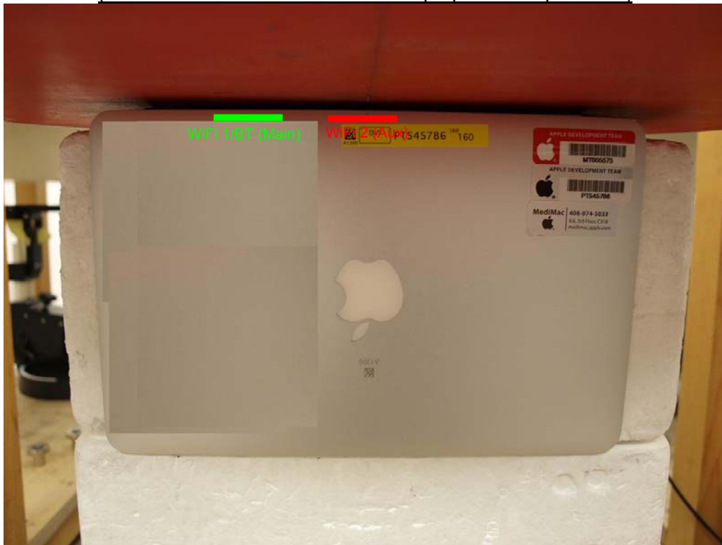
Nearby Person configuration for 11 inch MacBook Air (w/ 2.0 cm from back of the screen-to-phantom)
