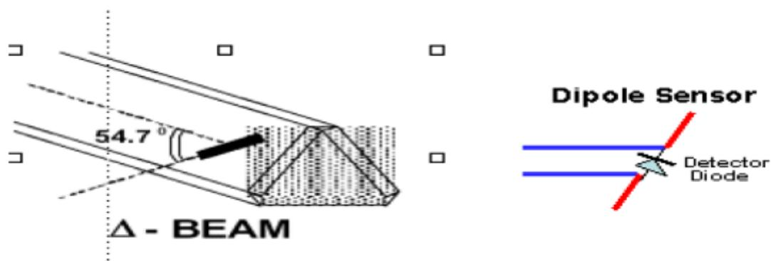
SAR is assessed with a calibrated probe which moves at a default height of 5mm from the center of the diode, which is mounted to the sensor, to the phantom surface (in the Z Axis). The 5mm offset height has been selected so as to minimize any resultant boundary effect due to the probe being in close proximity to the phantom surface.
