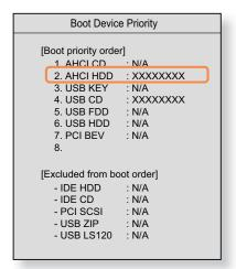
Press the F10 key to save the settings and exit Setup. The highest boot priority device is now set to the Hard Drive.
