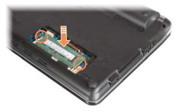
5 Close the memory compartment cover and fasten the screw.
