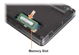
4 Push the memory module down so that it is completely fixed. If the memory does not fit easily, push the memory module down while pulling the memory module latches outward.
