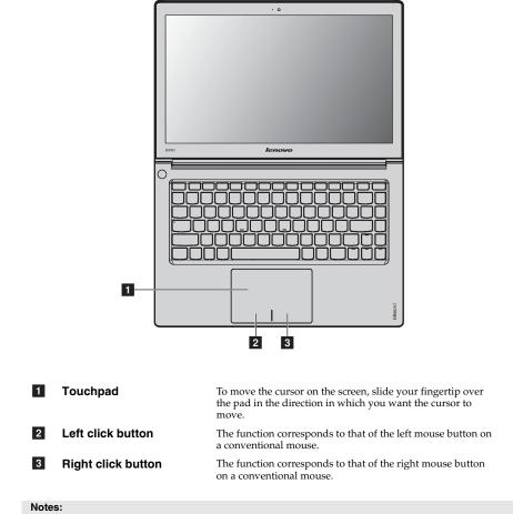
You can enable/disable the touchpad using **Fn+F6**. When the touchpad indicator is lit, the touchpad is disabled. •
