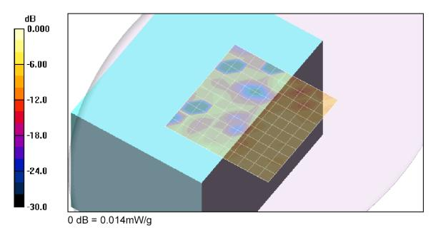
Maximum value of SAR (measured) = 0.014 mW/g
