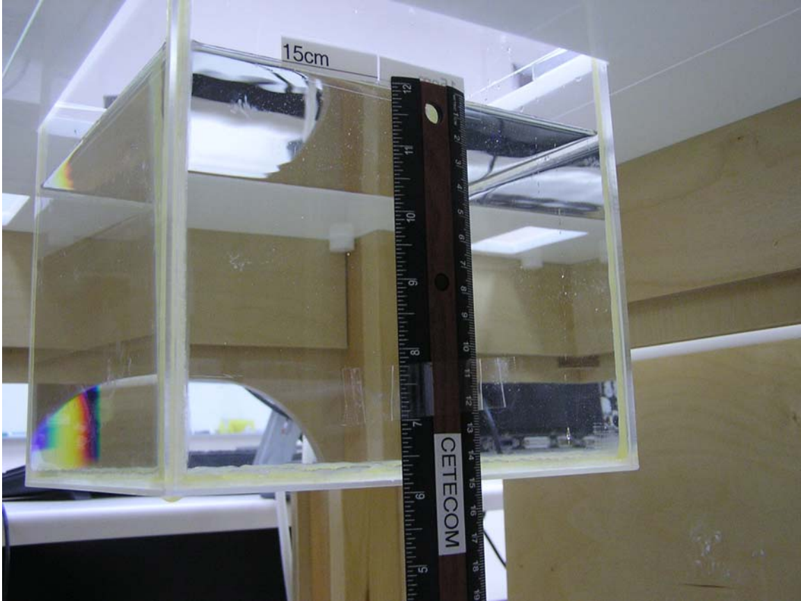
Photo 2. Photo to demonstrate 15 cm Z-axis flat phantom
