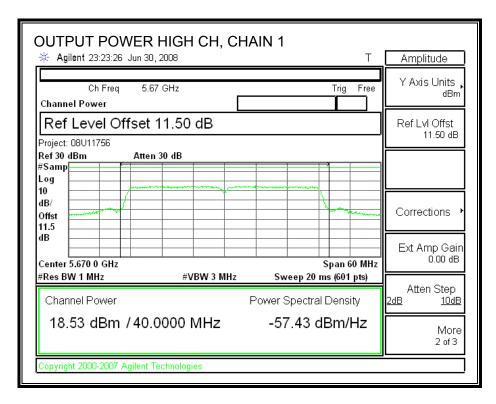
Antenna Combination: Hi PIFA / Low Slot = 8.80 dBi
