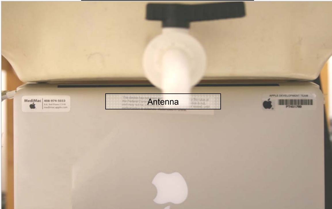
Setup Photo with SAM Phantom (2.4 GHz band)
