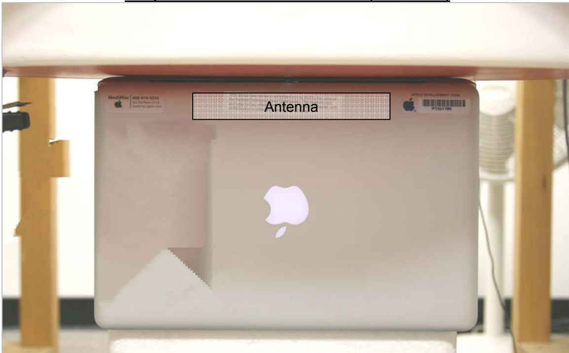
Setup Photo with Flat ELI 4.0 Phantom (5 GHz band)
