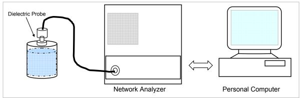
Set-up for liquid parameters check
