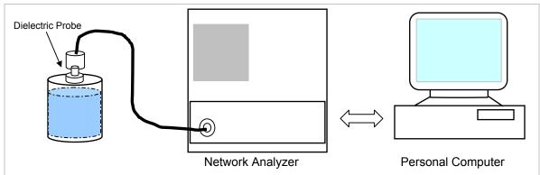
Set-up for liquid parameters check
