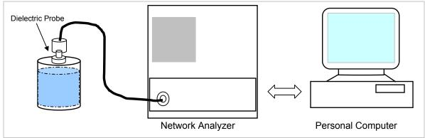
Set-up for liquid parameters check
