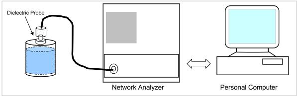
Set-up for liquid parameters check
