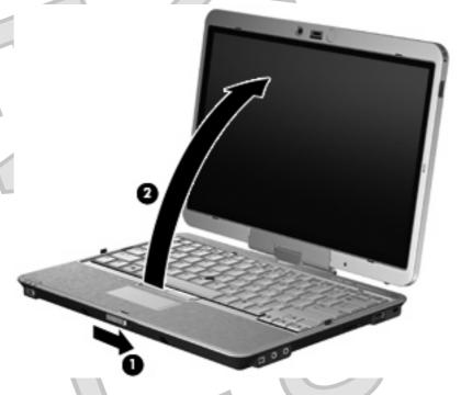
3. Rotate the computer display counterclockwise until it snaps into place facing the keyboard.
