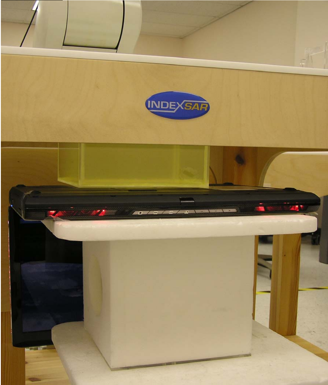
Photo 1. Auxiliary antenna, lap position
