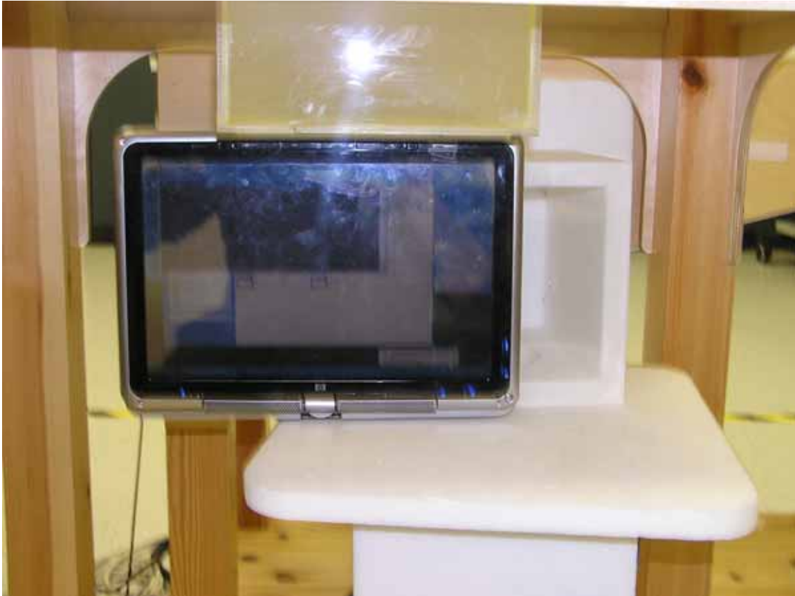
Photo 1. Tablet position, main antenna, top side
