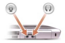
Attach a microphone to the  $\Theta$  connector. Attach headphones or speakers to the \(\infty\) connector.
