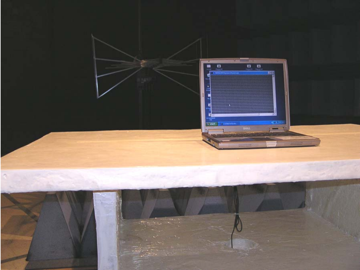
Test setup – Radiated Emissions
