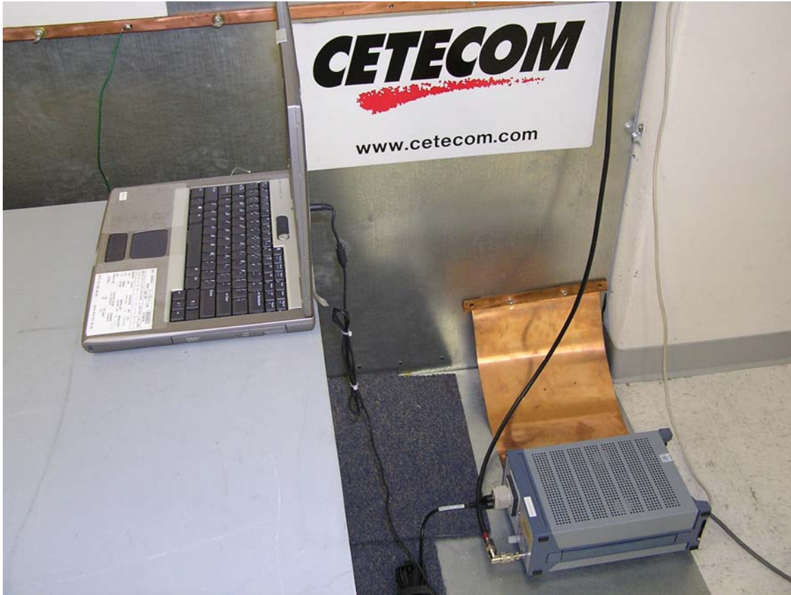
Test setup – AC Line Conducted Emissions
