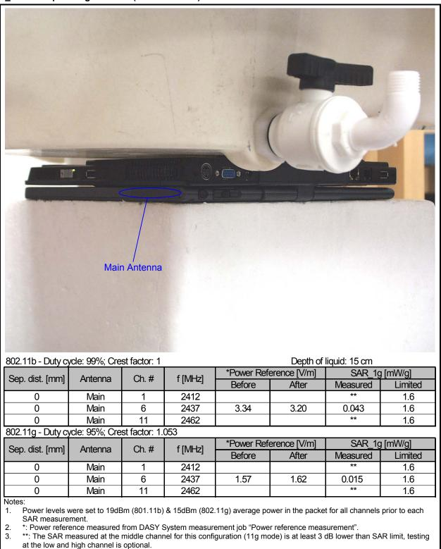
4. Host device is tested in a lap-held position with the bottom of the computer in direct contact against a flat phantom.
