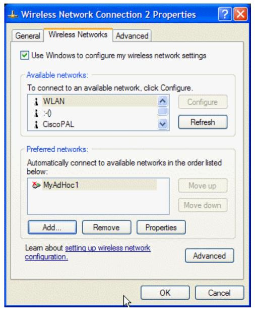
10. Reopen the **Network Properties** box and click the **Wireless Networks** tab. Your computer is connected to the added network when you see a blue bubble on top of the icon for your ad hoc network.
