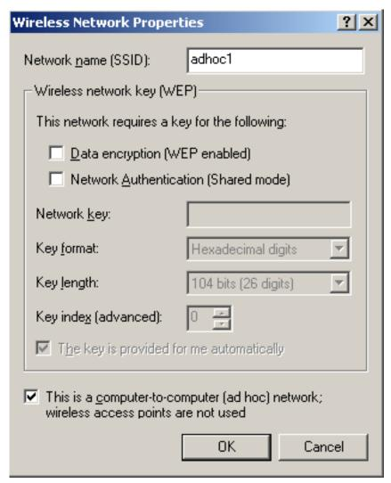
7. Click **OK** on the **Dell TrueMobile 1400 Internal Dual-band WLAN Card Utility** box to activate the ad hoc network (wait up to 1 minute for the network connection to be made). To verify that your computer is connected to the added network, reopen the **Dell TrueMobile 1400 Internal Dual-band WLAN Card Utility** and click the **Wireless Networks** tab. If you see a
