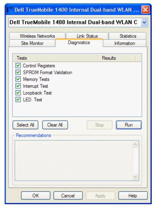
6. If your **Dell TrueMobile 1400 Internal Dual-band WLAN Card** fails any of the diagnostics tests, see the <u>Troubleshooting</u> section.
