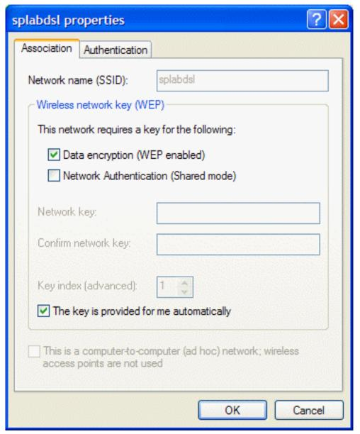
6. From the **Properties** box, you can enable or disable WEP data encryption and change the network name and the network key (see the <u>Completing the setup</u> section for instructions).
