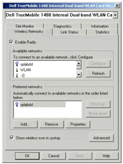
4. From the **Wireless Network Properties** box, you can enable or disable WEP data encryption and change the network name and network key (see the <u>Completing the setup</u> section for instructions).
