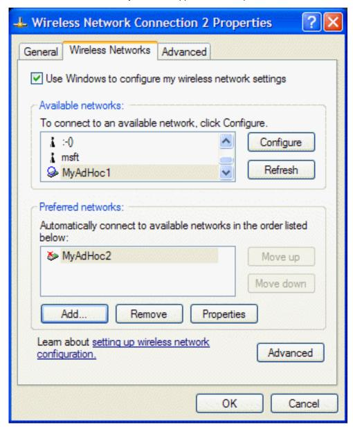
13. Reopen the **Network Properties** box and click the **Wireless Networks** tab. Your computer is connected to the added network when you see a blue bubble on top of the icon
