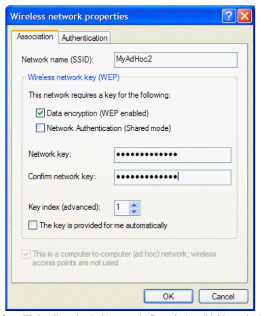
11. On the Wireless Networks tab of the connection Properties box, click Advanced, select Computer-to-computer (ad hoc) networks only, and click Close.
