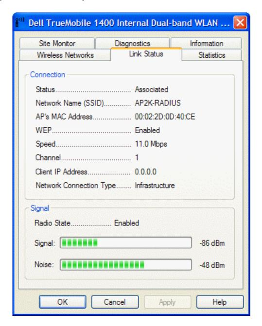
The quality of the connection (signal strength and noise) of the particular network you are connected to is indicated by the horizontal green bars and the decibel level values that are displayed at the bottom of the **Link Status** tab. The connection quality is also indicated by the appearance of the **TrueMobile 1400 Client Utility** icon in the desk top system tray. The verbal description of the signal strength appears when you hover the cursor over the icon.
