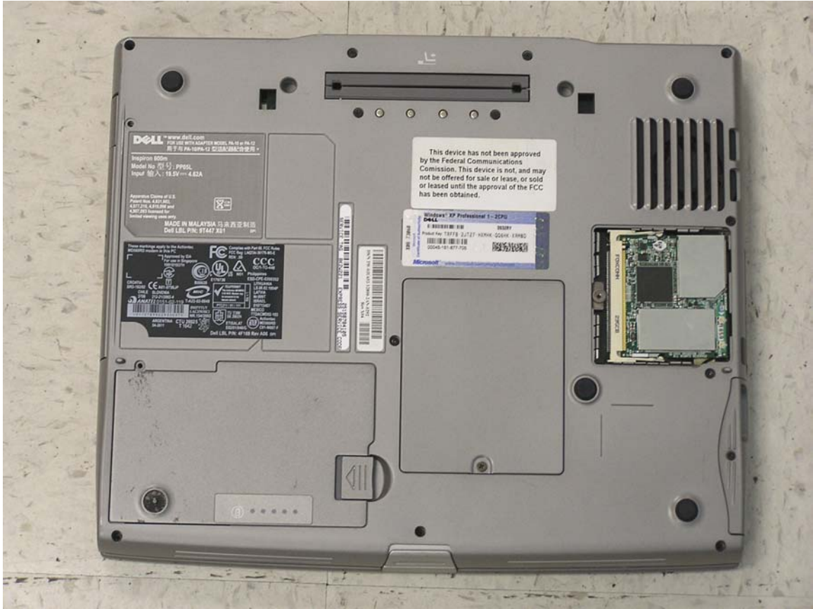
PP05X bottom view showing WLAN
