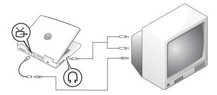
To connect the computer to a television that has a composite video input only, Dell provides a composite TV-out adapter cable. Before you begin, ensure that you have the following cables:
