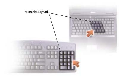
The numeric keypad functions like the numeric keypad on an external keyboard. Each key on the keypad has multiple functions. The keypad numbers and symbols are marked in blue on the right of the keypad keys.
