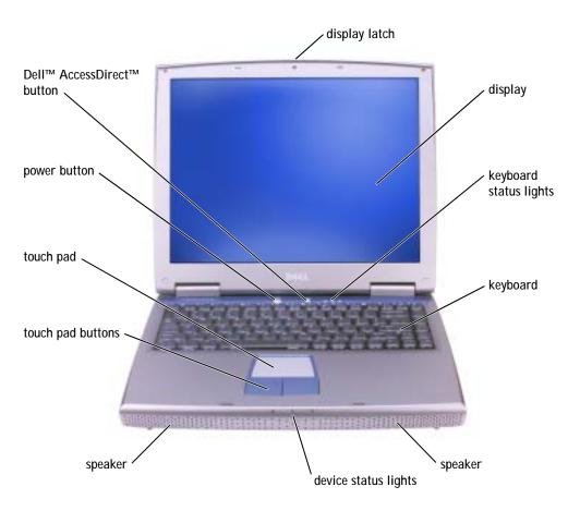
DISPLAY LATCH — Keeps the display closed.
