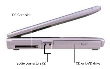
PC CARD SLOT — Supports one PC Card, such as a modem or network adapter. The computer ships with a plastic blank installed in the slot. For more information, see "Using PC Cards" in the Tell Me How help file. To access the help file, see page 74.
