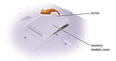
3 Remove the screw labeled "O" next to the memory module cover.
