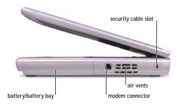
BATTERY/BATTERY BAY — When a battery is installed, you can use the computer without connecting the computer to an electrical outlet. See page 41.
