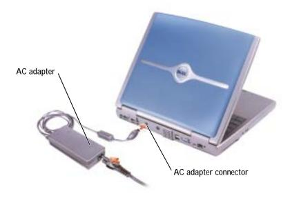
The AC adapter converts AC power to the DC power required by the computer. You can connect the AC adapter with your computer turned either on or off.
