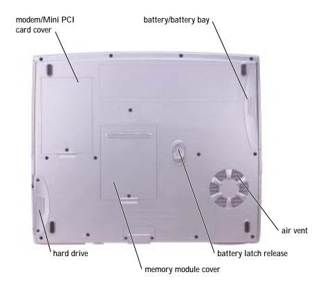
MODEM/MINI PCI CARD COVER — Covers the compartment that contains the modem and Mini PCI card. See page 96.
